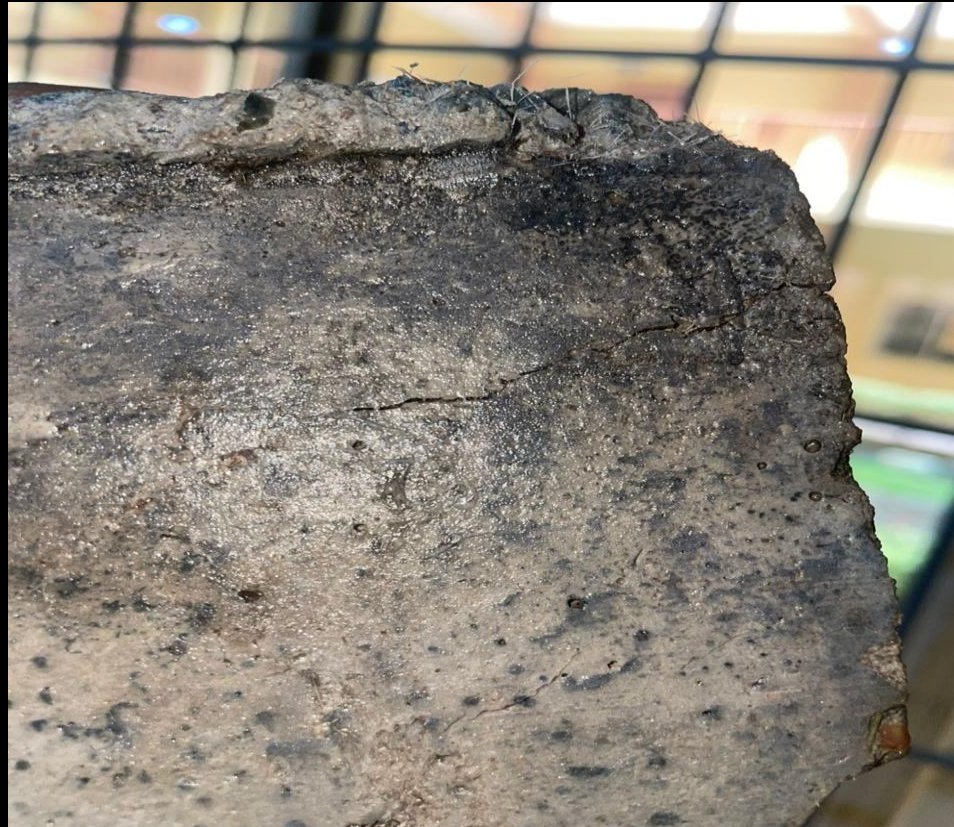
Figure 2: Visual inspection (initial crack stage)
